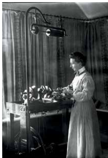
Lady Gertrude Crawford with her Holtzapffel ornamental lathe, fitted with an electric motor.
